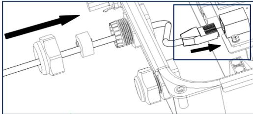
5. Connect the inverter to ZeverCom/ZeverManager or another communication device via the above- mentioned network cable.
