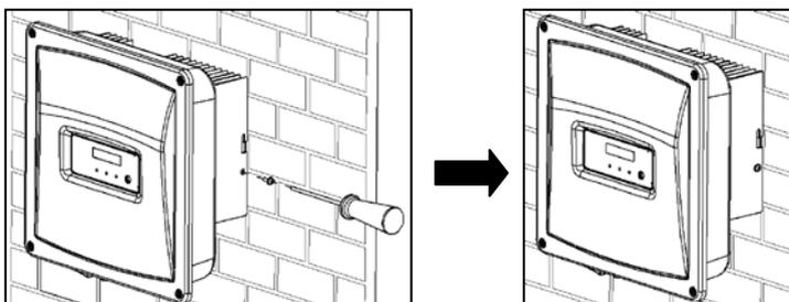
If a second protective conductor is required in installation site, ground the inverter and secure it so that it cannot be lifted off the wall bracket (see section 5.4.3 “Second protective grounding connection”).
