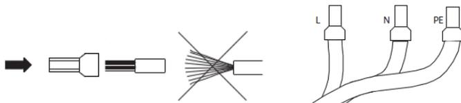
7. Connect the AC cable to the screw terminal block, using a flat-blade screwdriver (blade: 1×5.5) with a torque of 1.2 to 1.5Nm.
