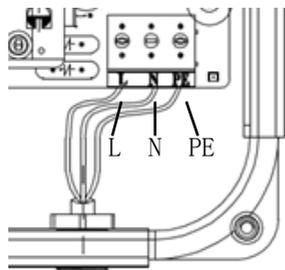
8. Make sure the insulated conductors are securely connected.
