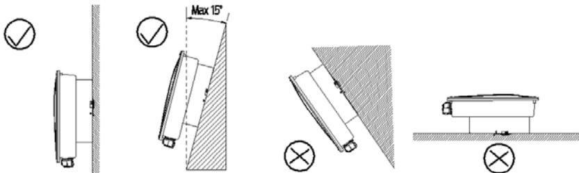
1. Mount the inverter vertically or tilted backward by a maximum of 15°.
