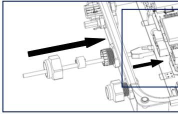
If the inverter has integrated ComBox (with Ethernet module), you need to insert the network cable into the RJ45 keystone socket on the ComBox.
