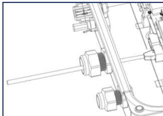
7. Secure the cover (torque: 2.2 - 2.5 Nm) using a screwdriver (T25).
