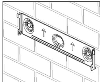
3. Holding the inverter and attach it tilted slightly downwards to the wall bracket.
