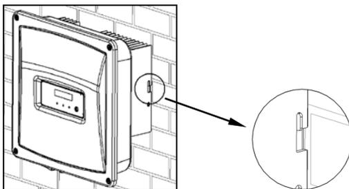
5. Push the inverter as far as possible and attach it to both sides of the wall bracket using the M5 screws.
