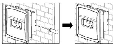
If a second protective conductor is required in installation site, ground the inverter and secure it so that it cannot be lifted off the wall bracket (see section 5.4.3 "Second protective grounding connection").
