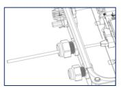
7. Secure the cover (torque: 2.2 - 2.5 Nm) using a screwdriver (T25).
