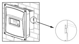
5. Push the inverter as far as possible and attach it to both sides of the wall bracket using the M5 screws.
