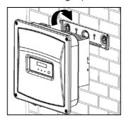
4. Check both sides of the heatsink to ensure that it is securely in place.
